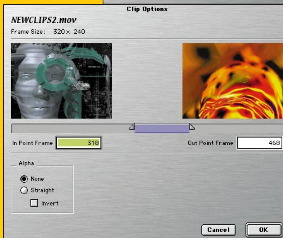
These dialog boxes are for beginning a new project (upper) and for importing a clip (lower). In the new project dialog, you set the frame size, the duration of the entire project and the quantity of frames to be loaded in to RAM for realtime playback. It's also possible to set the option to paint on fields. In the clip options dialog, in and out points are set, as well as alpha channel information.
