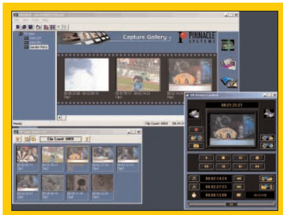
The DVTools interface. In this screenshot, one tape gallery is open, and a clip has been selected for viewing with the Device Control Window.
